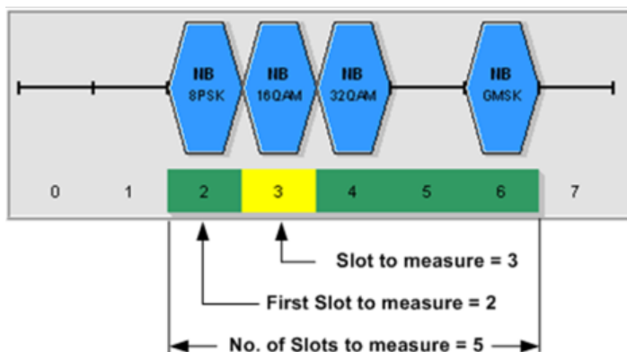
Fig. 4-21: Concept of "First Slot to measure", "Number of Slots to measure" and "Slot to Measure"
