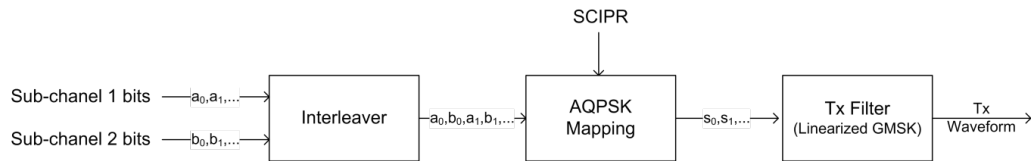
Fig. 4-19: AQPSK modulation scheme for GSM systems
